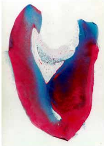
Porous sintered HA filled in prepared pulpal cavity of human wisdom tooth
